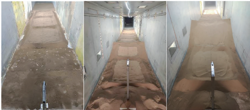
图 2 输沙量与沙障内蚀积状况测定 Fig. 2 Measurement of sand transport amount and erosion-deposition conditions within sand barriers
